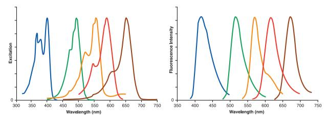
**Figure 1.** – Excitation (left) and emission (right) spectra of DyLight<sup>®</sup> fluorescent dyes conjugated to affinity-purified secondary antibodies. This figure illustrates the relative shape and position of each fluorophore in the peak area of its excitation and emission after antibody conjugation.
